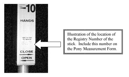
There are two parts to the measuring stick. The upright portion, with metric on one side and hands/inches on another side, has an extender that locks with a twist of the wrist. The cross bar has two levels to ensure accuracy of stick placement.
